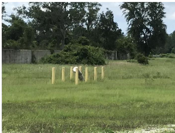
One end of a monitoring well drilled at an angle across the LCP site to assess groundwater contamination.
