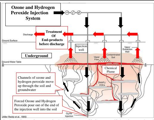
The chemical removal system at the site injects ozone and hydrogen peroxide into the contaminated groundwater and as they move up through the soil, they react with Site chemicals and break them down into less toxic end-products. The end-products are removed from the groundwater and then discharged into a well found within the slurry wall. The chemical plume is a high concentration of chemicals in a given area. Black = injection chemicals; Red = removed end-products from the chemical plume
